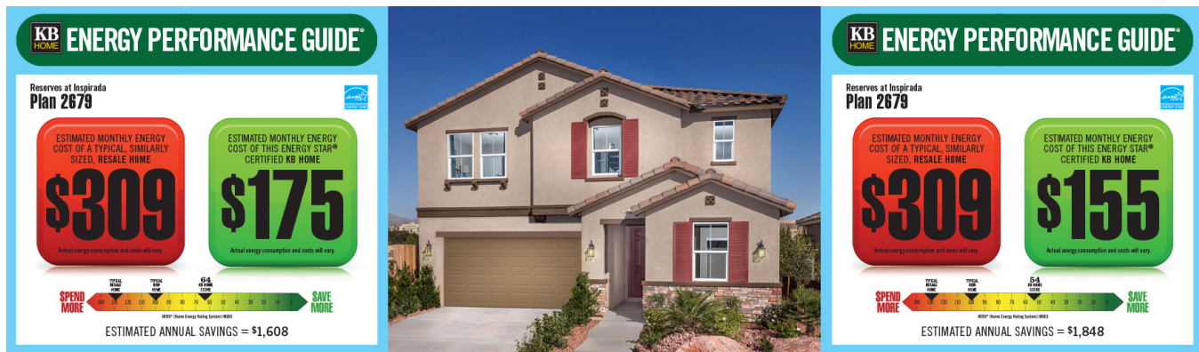
EPG for Plan 2679 before upgrade (left) vs. after (right) shows measurable result of upgrade to ENERGY STAR Version 3.1 in Las Vegas
